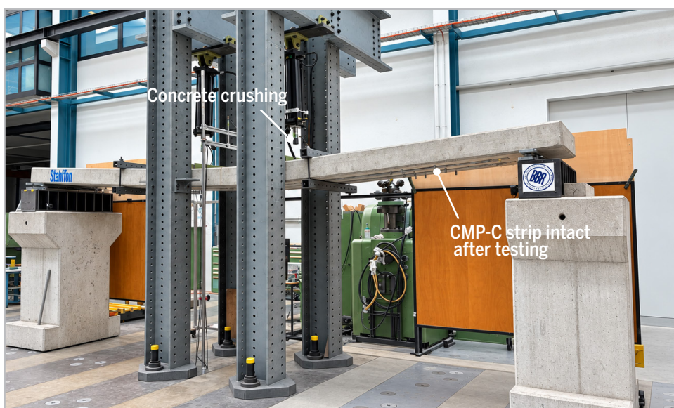
RC slab flexural test with CMP-C, sample after test
