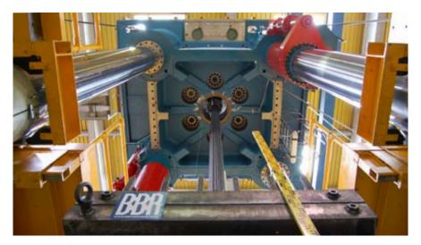
Although well in excess of the ETAG requirements, the team decided to go above eight million load cycles – already over four times more than required – in one additional voluntary test run. It was amazing that, even under these extremely hard conditions, the tendon endured this gruelling fatigue testing without any strands breaking.
