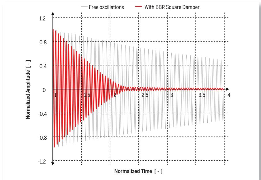
Figure 3. Time-displacement at the middle of the cable
