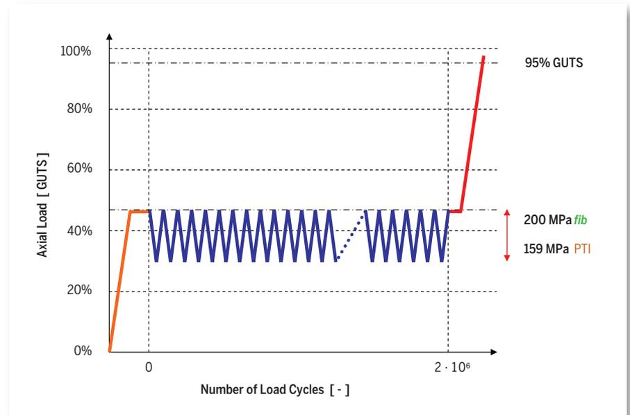
and in the order of 60% for applications with low fatigue demands (extradosed bridges). Loadings of stay cables during construction or cable replacement should not introduce inelastic deformations in the stay cable system, and a verification of axial stresses against permissible stresses is often sufficient. The permissible axial stresses during construction and cable replacement is typically limited to 60% – 70% GUTS.
