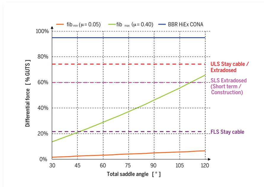
saddle – the BBR Saddle is a fixed structural point which ensures no-slippage and full load transmission between the stay cable and the saddle even under load scenarios that exceed the maximum permissible loads (i.e. 60% GUTS for accidental or short-term, according to *fib*). The BBR Saddle is proven by testing to transfer more than 95% GUTS.
