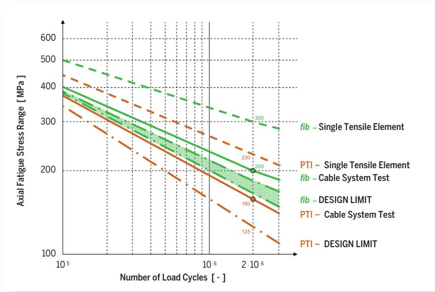
In an actual design situation, fatigue verification may need to be performed at a number of load cycles – other than 2 · 10<sup>6</sup> load cycles, where ‘Wöhler-Curves’ (S-N curves) can be used.
