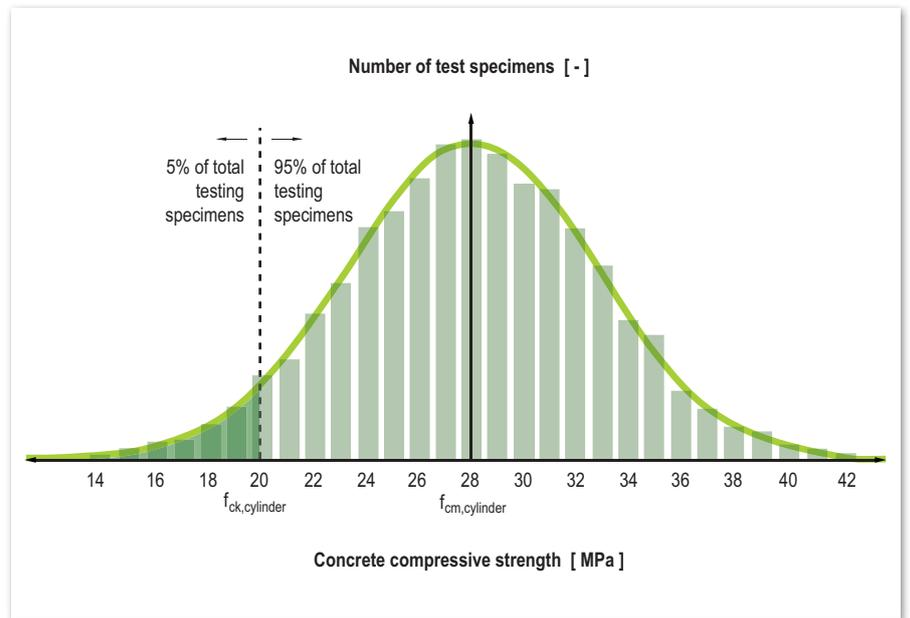
Figure 3: Generic normal distribution of concrete strength
