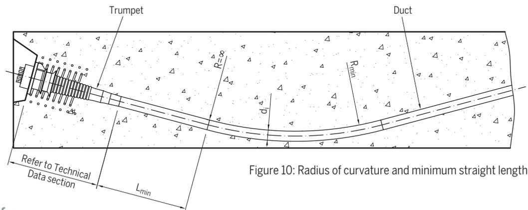
Figure 10: Radius of curvature and minimum straight length
