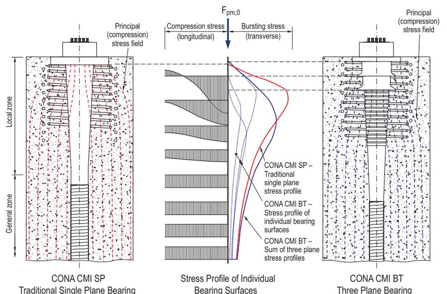
Figure 14: Stress distribution induced in concrete by a prestressing tendon
