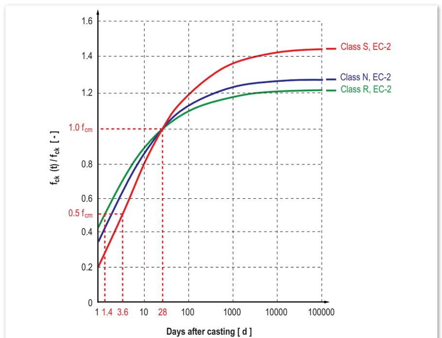
Figure 13: Concrete hardening
