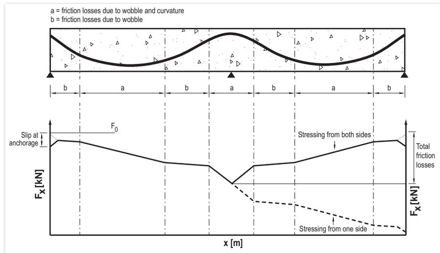
Figure 6: Concept of instantaneous losses
