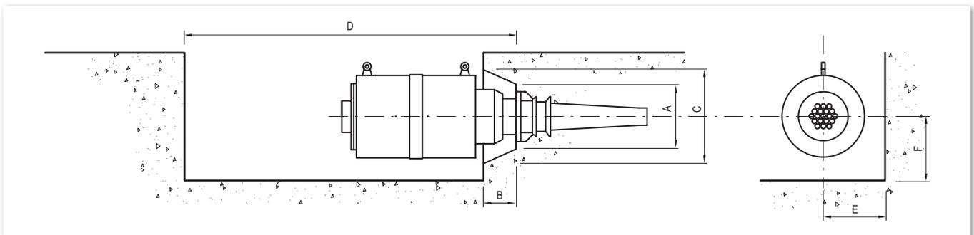
Figure 2: Dimensions of space requirements
