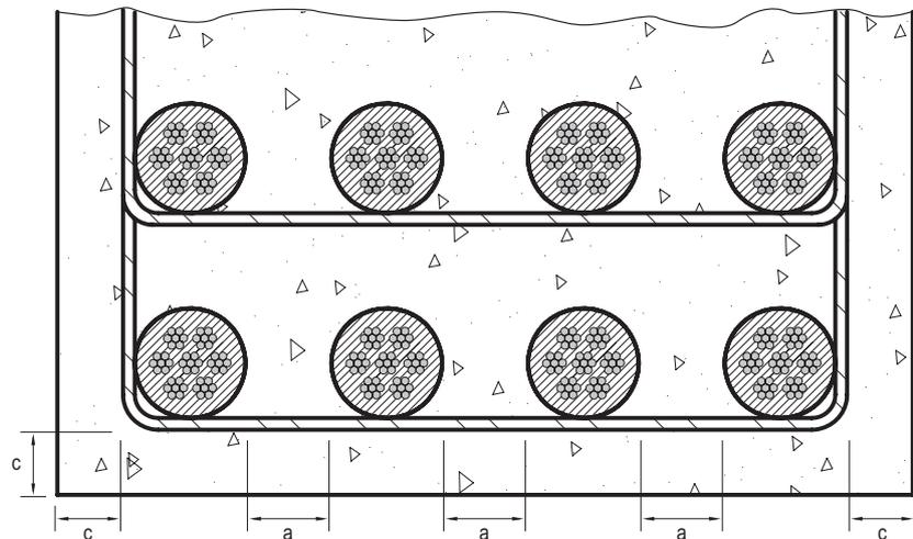
Figure 12: Tendon support on reinforcement and tendon layout
