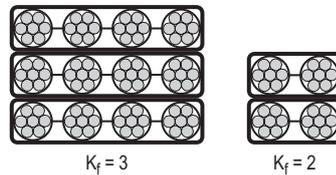
Figure 9:  $K_f$  factors in different strand configurations
