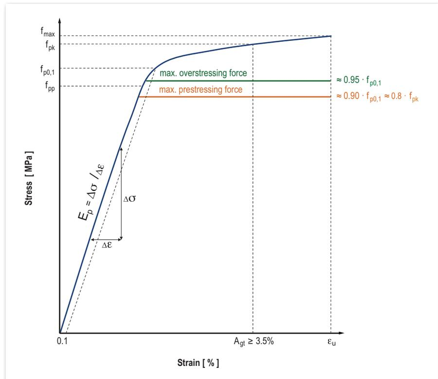
Figure 5: Stress-strain diagram of prestressing steel and relevant stress levels
