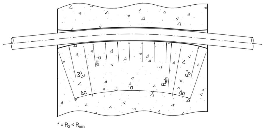
Figure 11: Minimum radius of curvature in deviators and saddles
