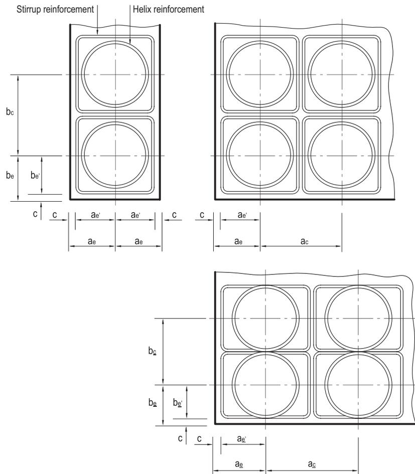
Figure 15: Dimensions of tendon center spacing and edge distance
