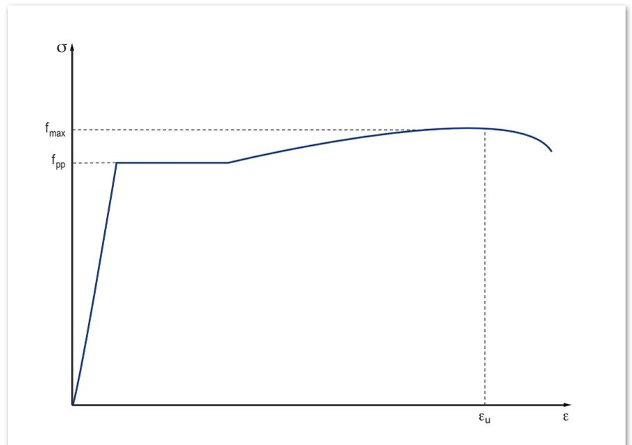
Figure 4: Stress-strain diagram of reinforcement steel
