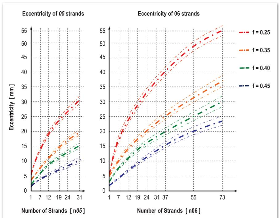
Figure 8: Eccentricity of 05 and 06 strands in a round duct
