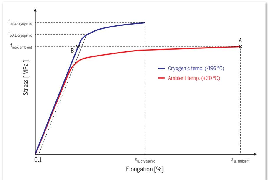
Figure 1: Static tensile test results comparing post-tensioning strands at different temperatures
