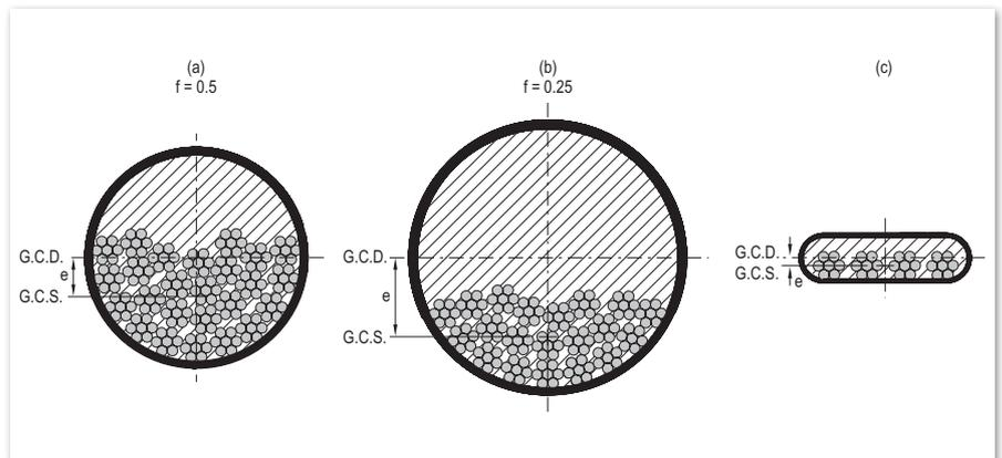
Figure 7: Center of gravity by high (a) and low (b) degree of filling of round ducts and flat duct (c)
