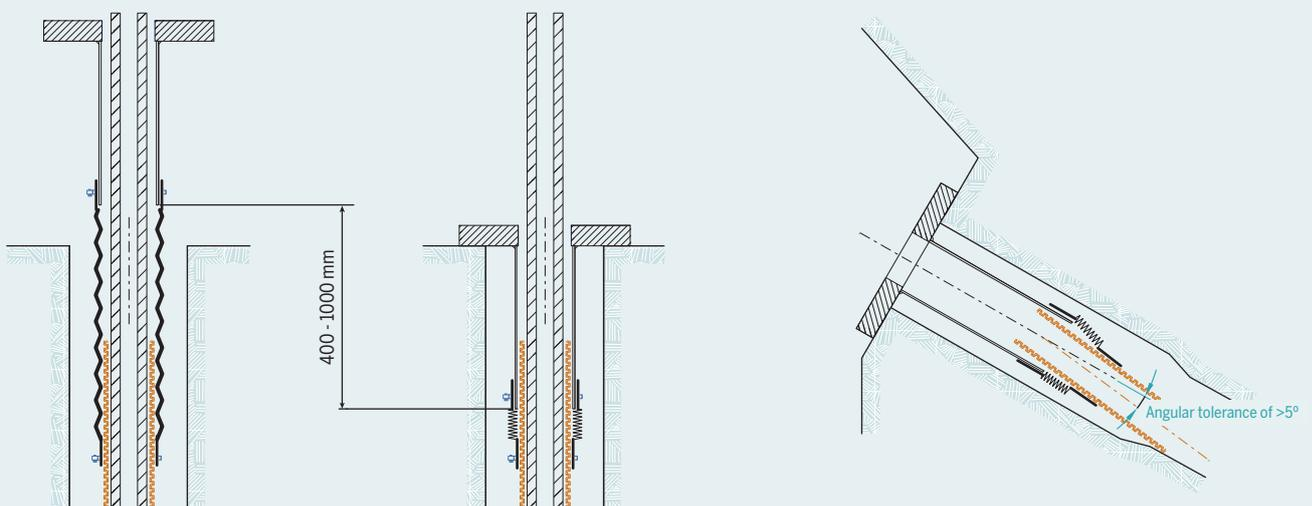
Schematic diagram showing the range of flexibility and tolerance built into CONA CMG’s unique sealing device for ease of installation on site.
