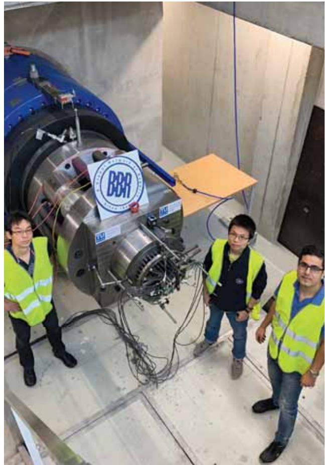
The high speed resonant testing facility for stay cables – which is frequently used by BBR VT International – is a great example of where innovation has been swiftly applied.
