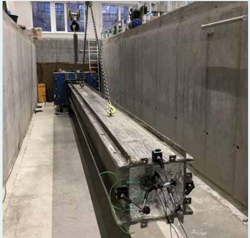
BBR’s extensive testing program according to the requirements of the EAD included an innovative test to prove the crack width of the inner cement grout under service load conditions – verifying that the grout acts as a corrosion protection layer.
