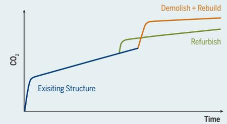
Carbon emissions generated by the demolition and rebuilding of an existing structure, as compared with its refurbishment.
