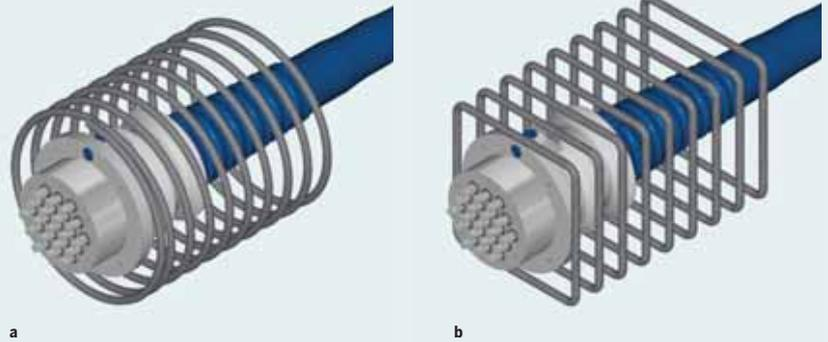
BBR solution for CONA CMI internal and CONA CME external post-tensioning systems – requiring only one layer of anti-bursting reinforcement, either helix (a) or stirrup (b).
