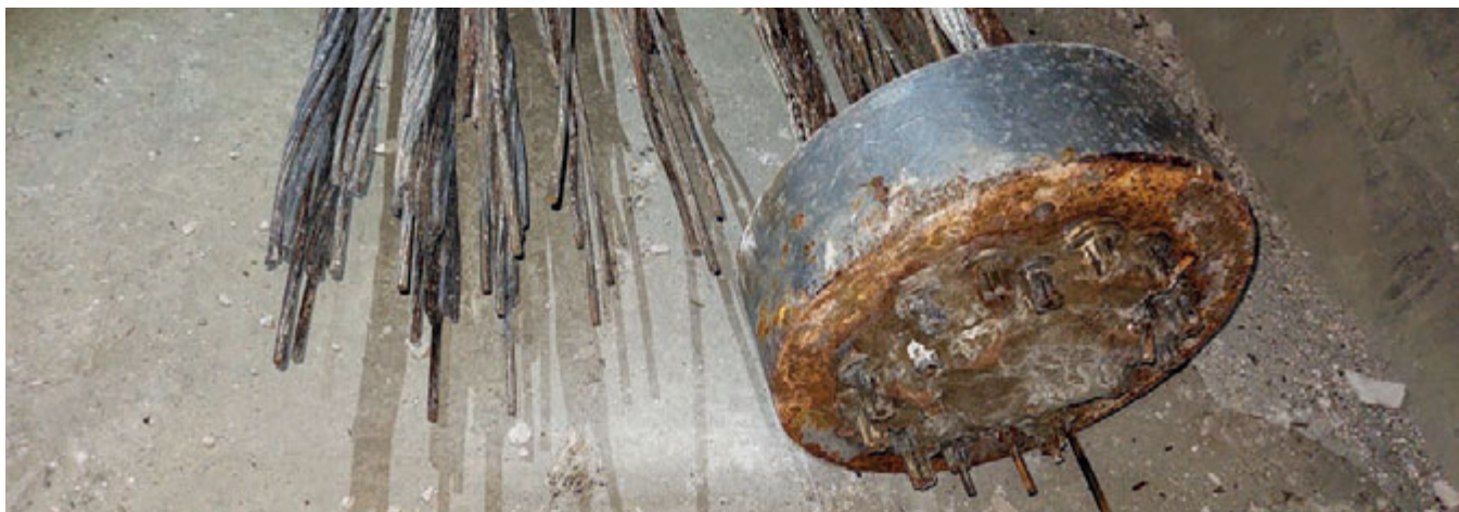
Localized electrochemical corrosion caused early PT tendon failure on a Vistula River Bridge. BBR Polska Sp. z o.o. applied BBR Care+ technologies to complete the repair and future safeguarding against corrosion.
